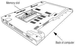
(Sample Illustration) Removing the memory module
